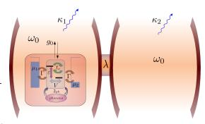
Coupled cavities with a voltage biased double-quantum-dot in one of them.
